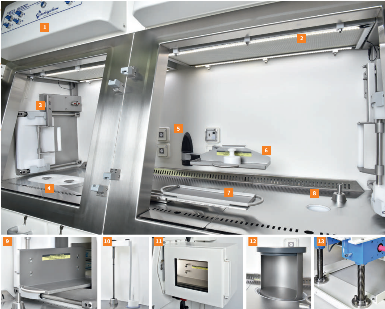
1 | Control panel 2 | Extra-large HEPA filters covering the entire work surface and LED lighting 3 | Manual opening system of the airlock chamber inner sliding door 4 | 2 generator access points 5 | Electrical, USB and RJ45 sockets 6 | Hinged shelf 7 | Sliding transfer tray 8 | Dose calibrator chamber access 9 | Airlock chamber sliding tray for transfer of accessories and consumables 10 | Pneumatic dipper raising system (optional) 11 | Lead glass lateral airlock chamber (optional) 12 | Front airlock chamber (optional) 13 | Electric hot cell lift (optional)
